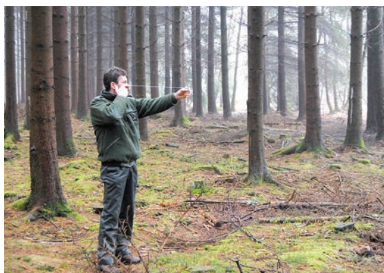
Measurement of the basal area with a notched Relascope (Beauraing, Belgium).
